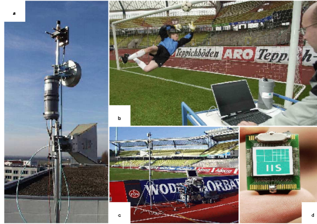
Fig. 1. Microwave-based position tracking system: (a) receiver; (b)&(c) installation; (d) sender.
