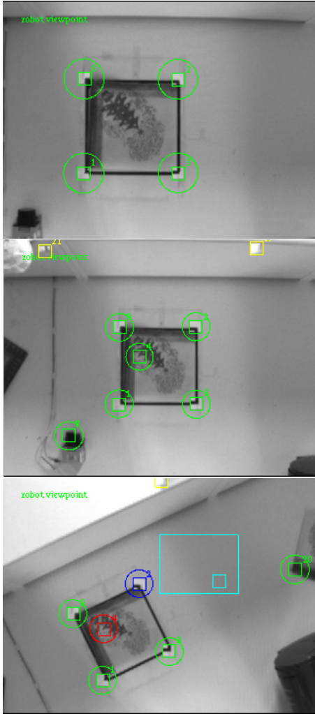
Figure 6. Top: Initial setup, robot 0.7m away from origin, Middle: Robot was translated 1m backward on z-axis, Bottom: Robot(camera) was rotated -30^\circ around z-axis. The world coordinate frame is in the center of the rectangle with x-left, y-up, z-forward
