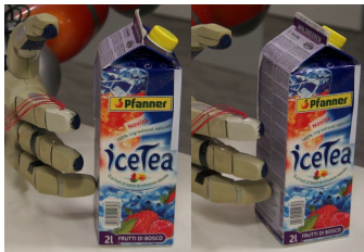
Fig. 1. TUM-Rosie robot pushing a box
