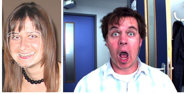
Fig. 2. Shape information is extracted to represent the state of various facial feature such as the rising of the eye brows or the opening angle of the mouth.
