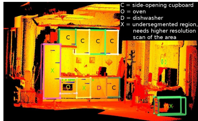
Fig. 2. A functional map of the kitchen environment superimposed on the raw scan from which it was obtained.
