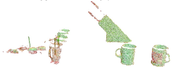
Fig. 8. Example of triangulated surface models for a few raw point clusters show in intensity (red shades).
