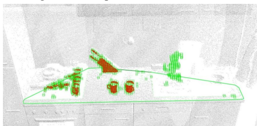
Fig. 10. Object clustering based on octree connectivity segmentation on a planar horizontal surface (i.e. table). Only points in red are selected as object candidates, as the rest does not fulfill the object footprint criterion.
