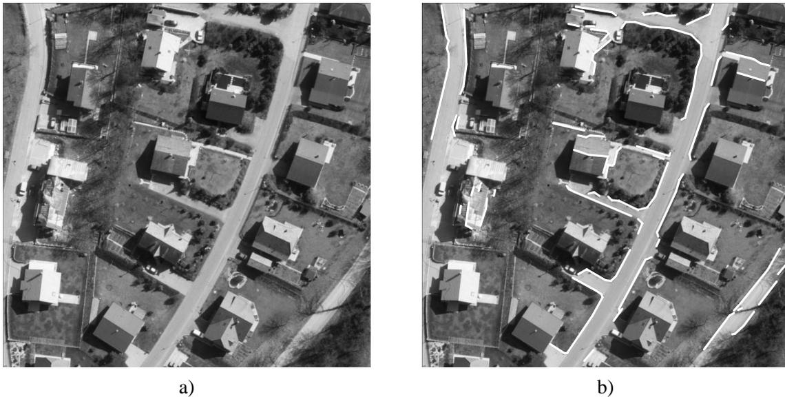
**Fig. 8:** a) Image 5897 of the Ascona testset b) Final result of the road extraction process
