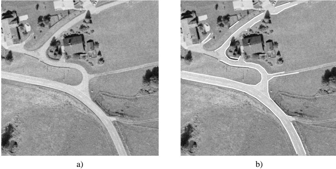
**Fig. 7:** a) Input image to the algorithm b) Final result of the road extraction process
