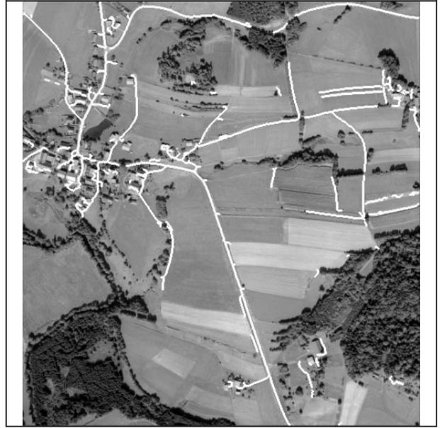
Fig. 2: Results of low resolution road extraction
