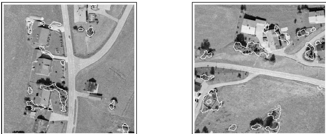
Figure 6. Classified pixels (class tree) after noise elimination.
