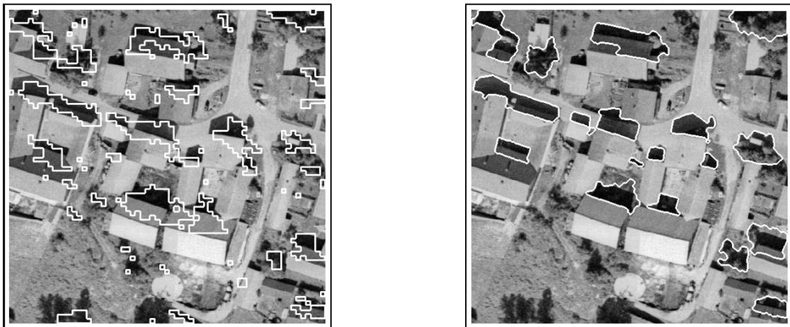
Figure 9. Raw segmentation after illumination of DTM (left) and after noise cleaning (right).
