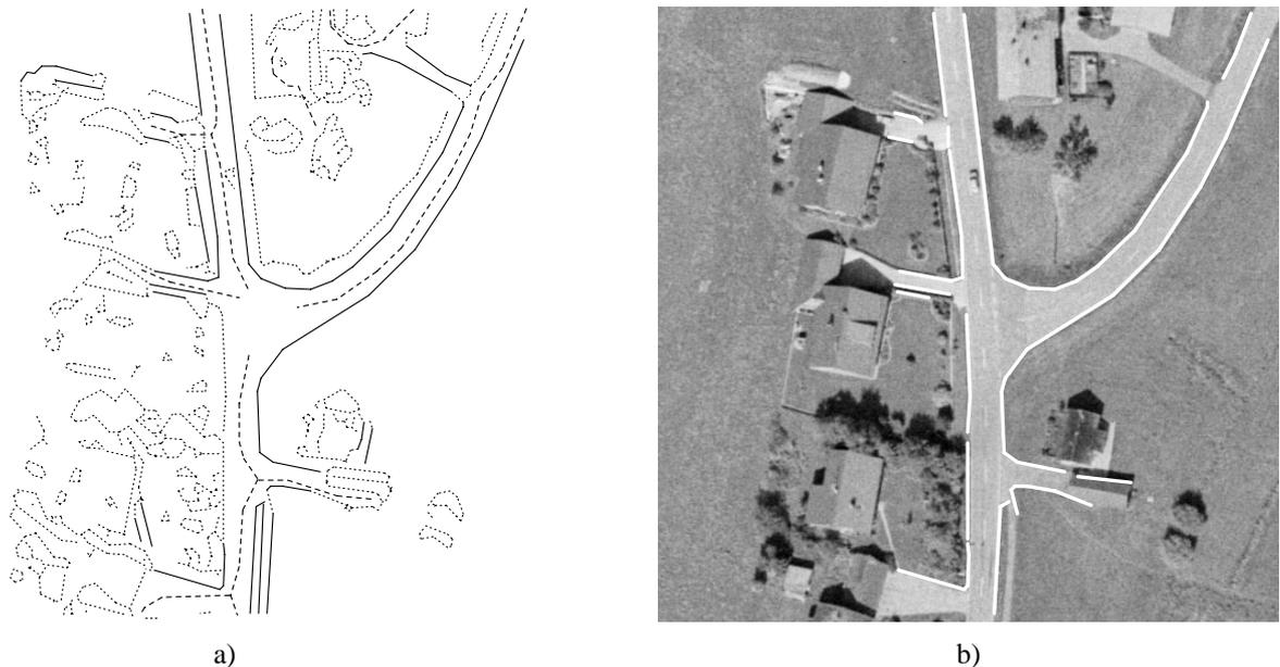
Figure 5. a) Input to the combination step b) Final result of the road extraction process
