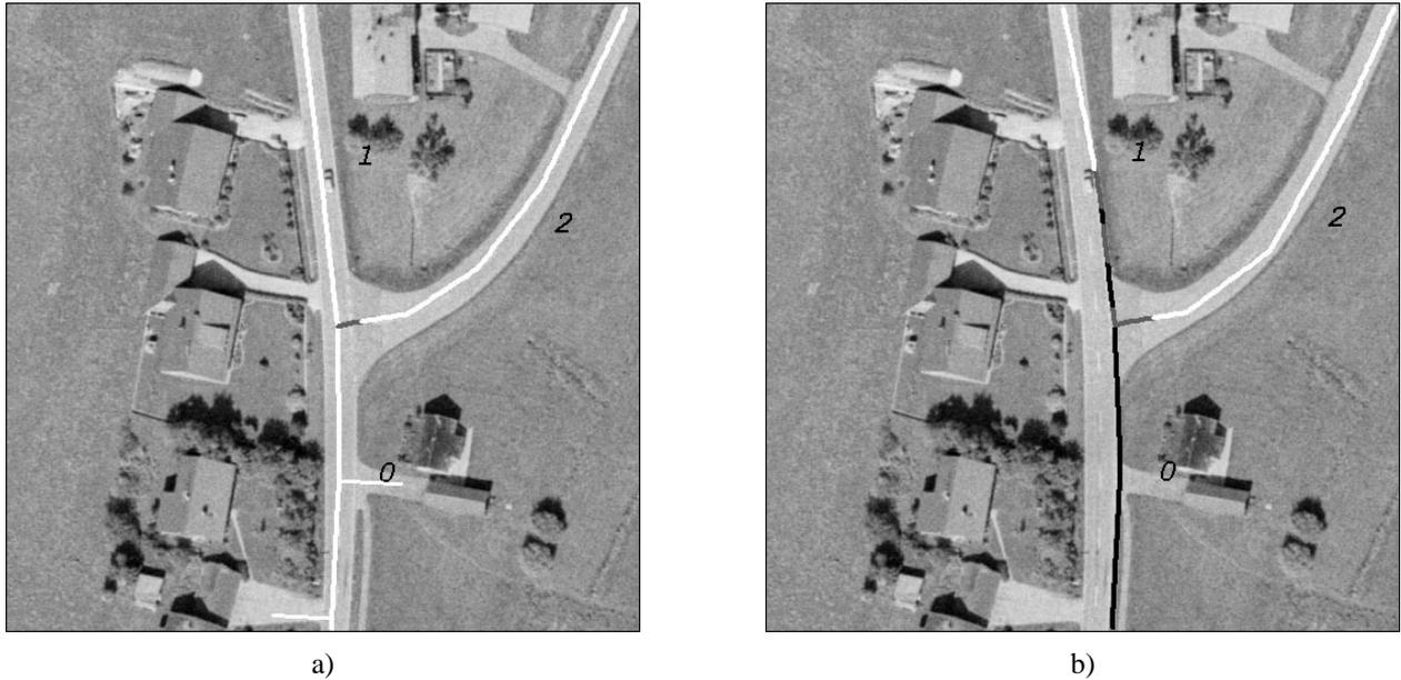
Figure 2. Results of verifying a) accurate and b) inaccurate GIS road axes
