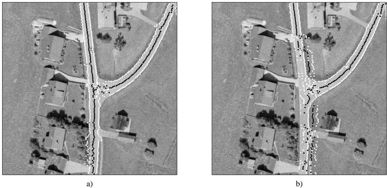
Figure 1. Extracted edge points a) for accurate and b) inaccurate GIS road axes (see Fig. 2
