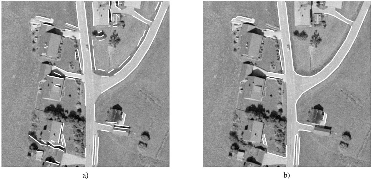
Figure 4. a) Detected parallel line segments b) Selected parallels that enclose a homogeneous region or are adjacent to one
