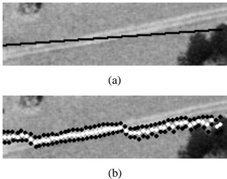
Figure 2: a) Inaccurate axis b) Skips in edge detection
