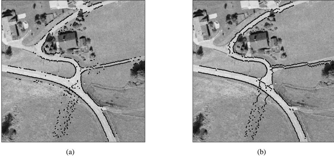
Figure 1: Edge points a) before and b) after the estimation of the road width
