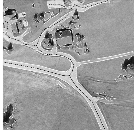
Figure 8: Input to the fusion: hypotheses for road axes (dashed, black), hypotheses for roadsides (solid, white) and other edges (dotted, white)
