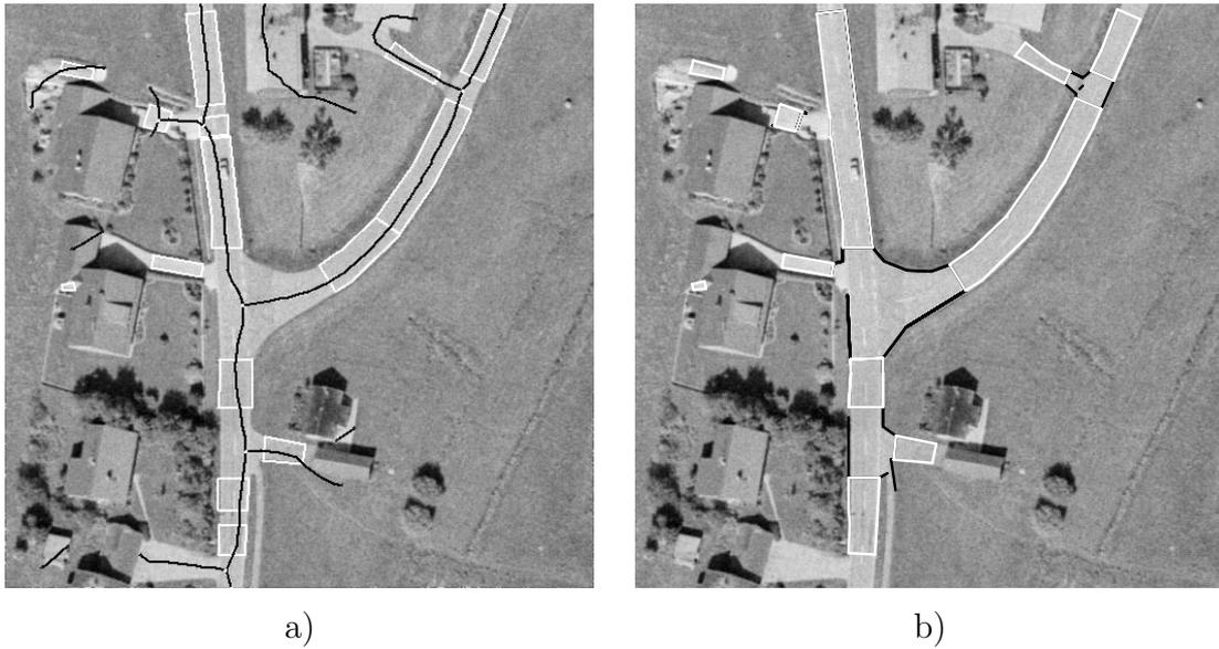
**Fig. 9:** a) Road-segments (white), lines (black) and junctions (white points). b) Polygons of intersection areas (black) and road-segments (white).
