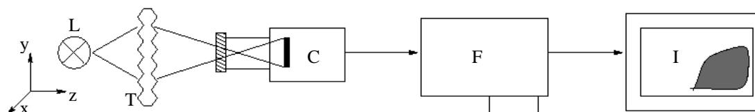
Figure 1: Schematic view of the arrangement (L: LED, T: cutting tool, C: camera, F: framegrabber, I: image processing)
