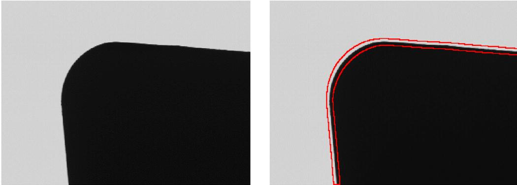
Figure 4: Image of a cutting tool (left side) and region of interest for edge detection (right side, red)
