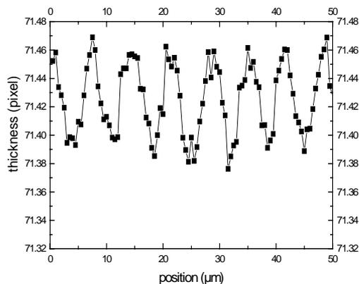
**Figure 9: Thickness oscillations of a stick measured over a distance of 50  $\mu\text{m}$**
