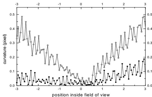
**Figure 3: Curvature of a vertical line before (upper curve) and after (lower curve) calibration**
