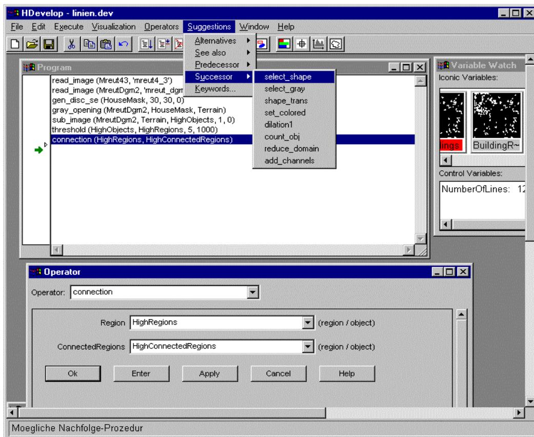
Figure 3: Suggestions menu for the connection operator
