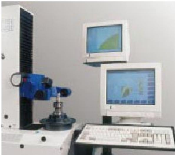
FIGURE 8: Machine for high precision measurements of tools with HALCON image processing
