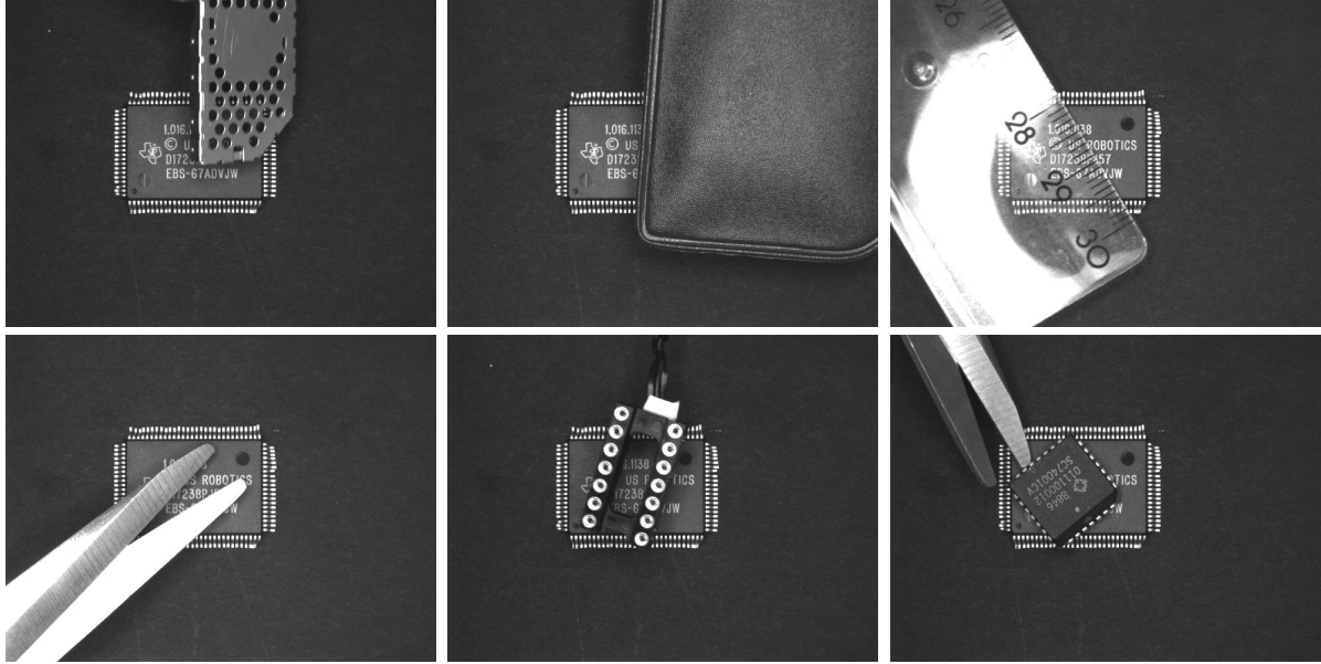
Figure 5. Six of the 500 images that were used to test the robustness against occlusions.
