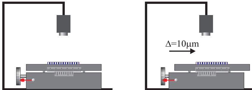
Figure 7: To test the accuracy, the IC was mounted on a precise  $xy\theta$ -stage, which can be shifted with an accuracy of  $1\ \mu\text{m}$  and can be rotated with an accuracy of  $0.7'$  ( $0.011667^\circ$ ).
