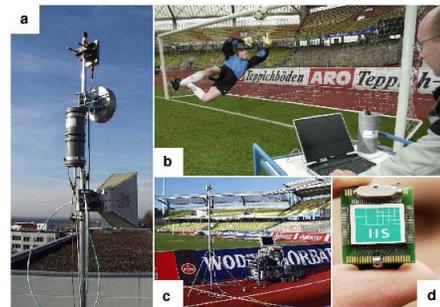
**Figure 1. Microwave-based position tracking system: (a) receiver; (b)&(c) installation; (d) sender.**
