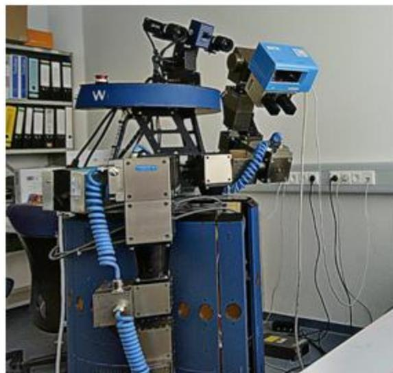
**Figure 1.** B21 robotic platform equipped with a SICK LMS 400 laser mounted on PowerCube arms.
