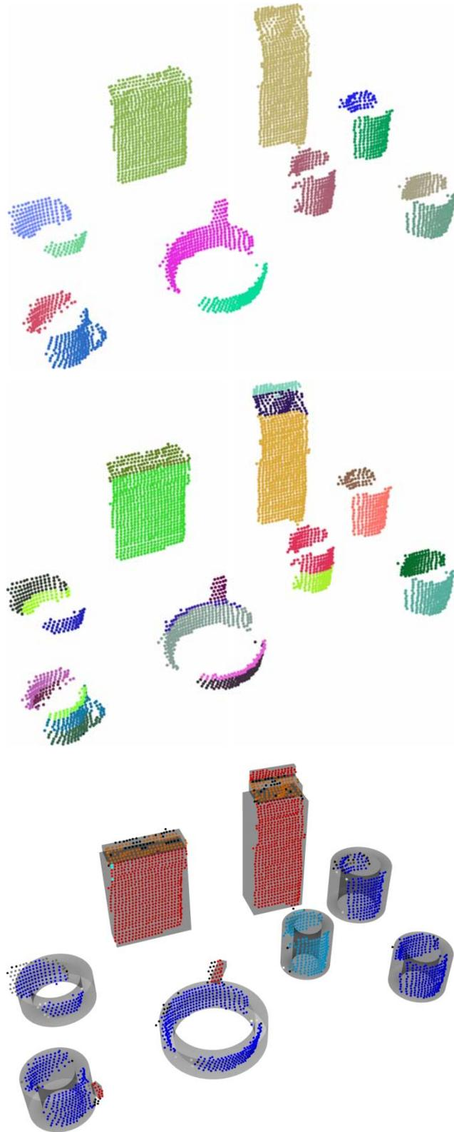
**Figure 2.** The basic steps of the algorithm illustrated from top to bottom: Extracting connected clusters of points from on top of a table’s plane, adaptive layering of each region, and reconstruction using shape primitives while dealing
