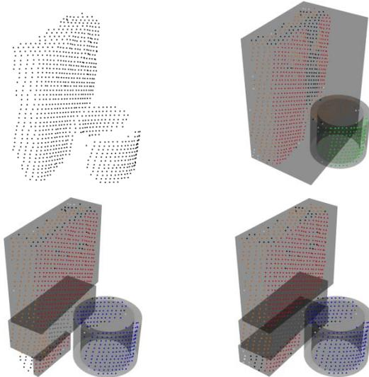
**Figure 4.** Dealing with under-segmentation, from left to right, top to bottom: a) two closely positioned objects which end up being clustered together; b) before using the splitting strategy; c) after using the splitting strategy; c) expanding the shapes in the occluded areas.
