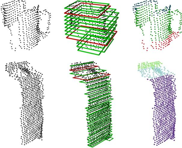
**Figure 3.** Example of a mug and a tetra pack decomposed into layers, from left to right, by columns: a) objects' point clouds from a single view scan; b) sliced regions into thin layers where red rectangles represent jumps; c) decomposed regions into adaptive layers.
