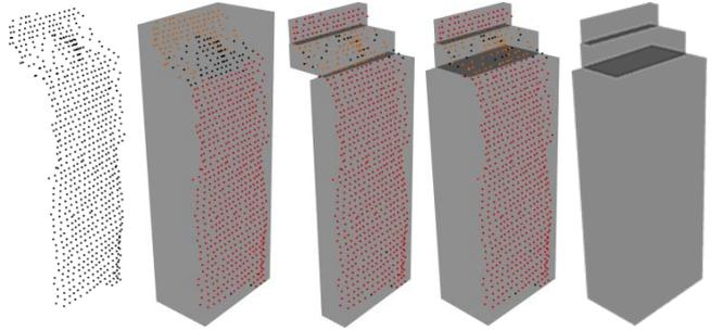
**Figure 5.** Example of reconstruction using box shapes, from left to right: a) scanned tetra pak; b) reconstruction before using layered decomposition; c) reconstruction after using the layering procedure; d) expanding shapes in the occluded areas; e) CAD-like model used for grasping.
