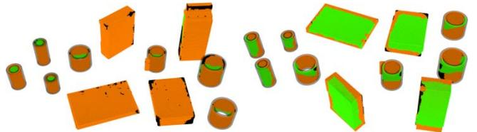
**Figure 6.** Verification of object models viewed from the upper-front (a) and lower-back (b). The orange points are marked as verified, green ones as invisible and the black points as void.
