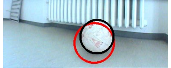
Figure 7: The mainly white non-RoboCup ball is accurately segmented in front of a white-grey background. This is hardly possible with color labeling (red: initialization, black: estimated ball contour).
