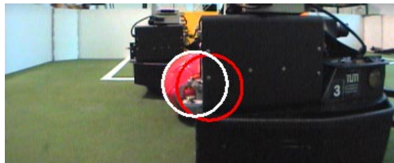
Figure 1: The proposed method correctly localizes the ball despite the partial occlusion. (red: initialization, white: estimated ball contour)
