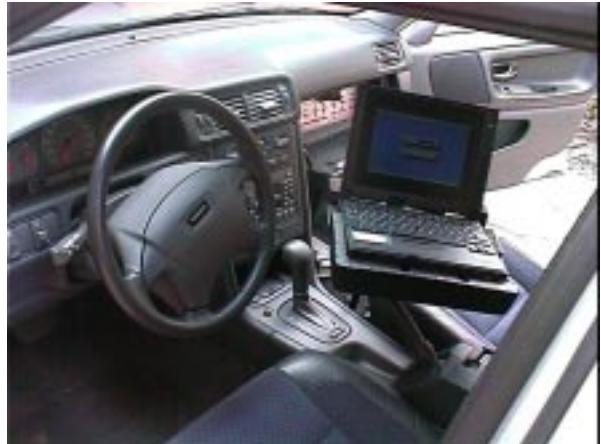
Fig. 5. View of the Volvo Demonstrator Car showing the notebook connected to the ECU. The glove compartment (behind) contains the switchboard for controlling the built-in faults.
